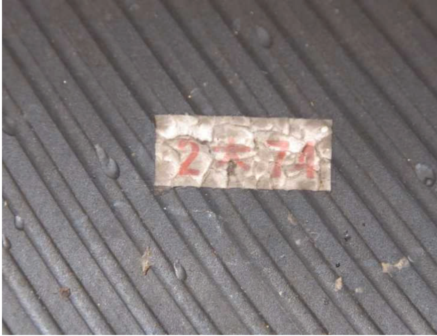
Innerliner sticker in tubeless tyre
