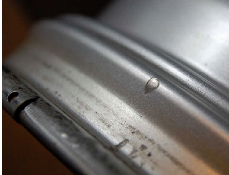
Damage on alloy tubeless rim from bead breaking tools, not good for tubes
