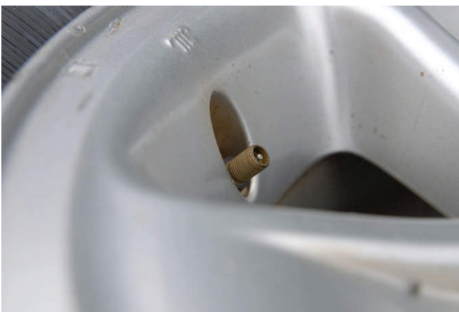
Tube valve barely poking through alloy rim
