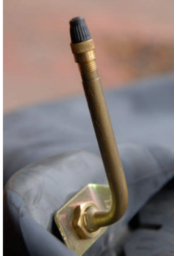
TR75A common split rim valve stem
