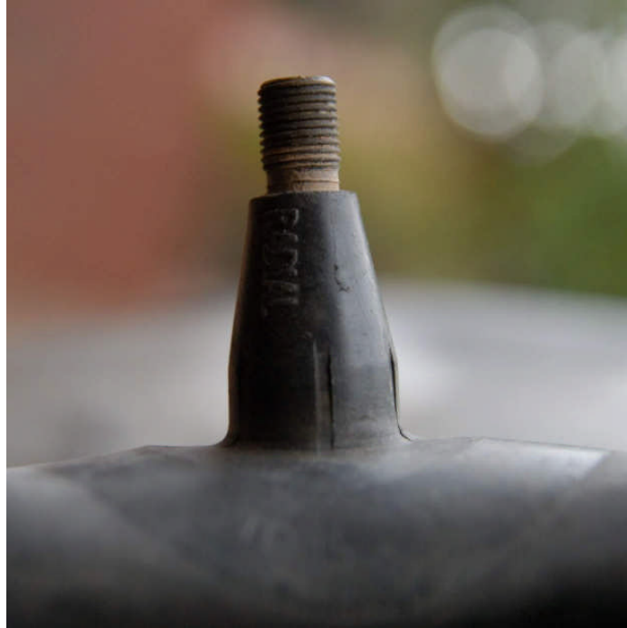
TR15 tube rim valve stem
